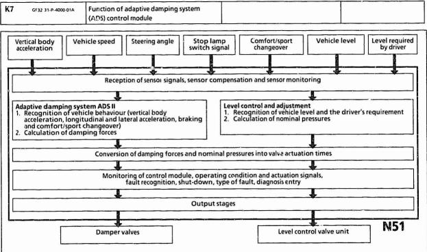
The adaptive damping system (ADS) control module is broken down into the following functions:
