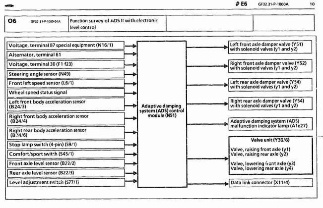
The corresponding functions of the hydraulic control circuit are controlled with the electrical/electronic components.
