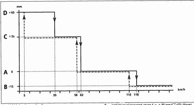
Vehicle level normal = 0 mm Vehicle level lowered = -15 mm
