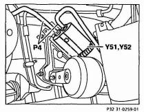
Y51 Left front axle damper valve Y53 Left real
