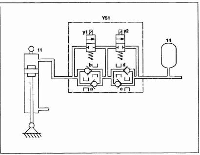
Four damping force stages can be achieved via the actuation of the adaptive damping system (ADS) control module.
