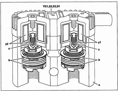
The damper valve (Y51, Y52, Y53, Y54) consists of the housing (a) and the 2-piston/reed valve packages (b). The spring-loaded (c) solenoid valve pistons and the solenoids in the upper section of the housing are located above these. The valve pistons and solenoids form the solenoid valve units (v1, v2).
