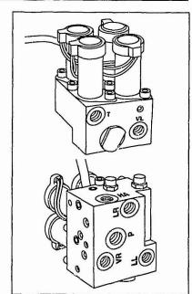
Level control valve unit Y36/6 Raising front axle valve Raising rear axle valve Lowering front axle valve Lowering rear axle valve Distributor valve Pressure relief valve Discharge valve Non-return valve Y51 Left front axle damper valve Right front axle damper valve Y52 Left rear axle damper valve Y53 Y54 Right rear axle damper valve Pressure oil pump Oil reservoir Rear spring actuator Rear spring strut Front spring strut 11
